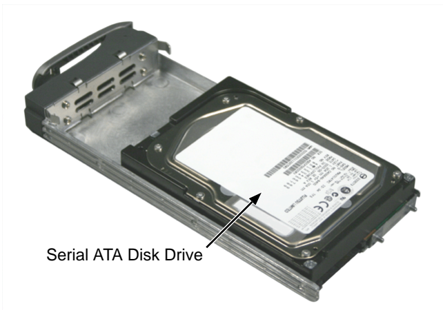
Figure 4. SATA Disk Drives mount at the front of the carrier
